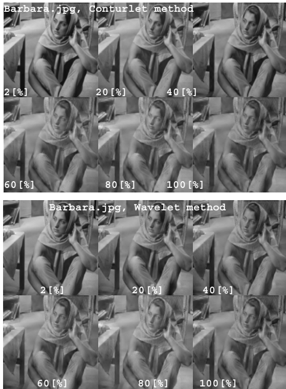
Figure 5: Sample images (Barbara.jpg) for contourlet and wavelet methods, different probability of distortion of individual "refinement bits" in sequence.
