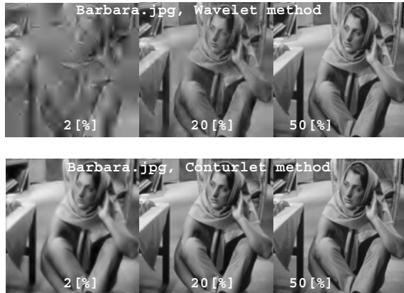
Figure 1: Sample images (Barbara.jpg) for contourlet and wavelet methods, after decoding 2[%], 20[%], 50[%] of the output SPIHT sequence.
