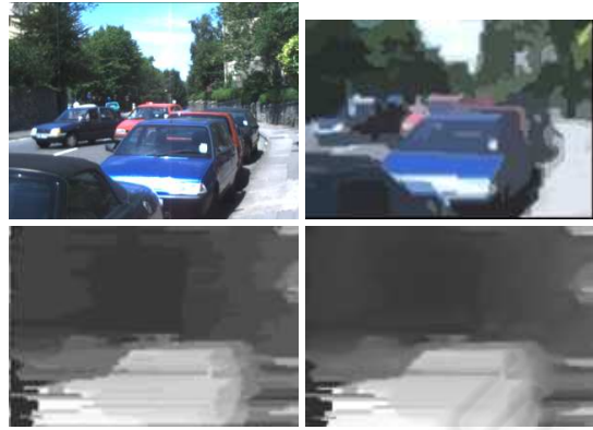
Figure 1: Fusion of depth map with image segmentation. 1st row: the original left image and graph cut based segmentation using colour and raw depth information; 2nd row: original depth estimation and result after anisotropic smoothing based on segmentation.
