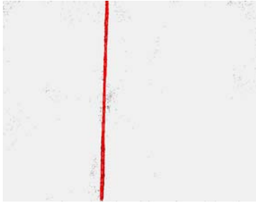
Figure 10: The trimap for Fig. 8a: red pixels are defect, light grey are non-defect and black are unknown (appear sparse and small in this case).
