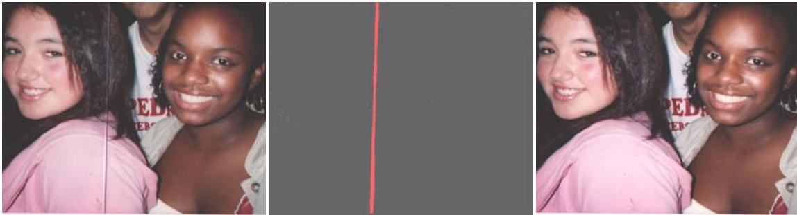
Figure 1: Left: Original scan of a damaged photograph. Middle: 3D structure present on the surface of the print extracted by our method. Right: Automatically repaired photograph using 3D structure information and infilling methods.
