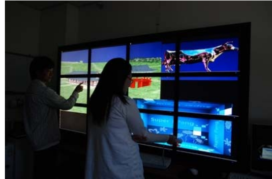
Figure 3: Users interact with three iTILE applications on the 4x3 iTILE tiled display system.
