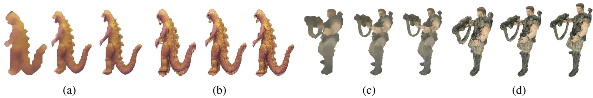
Figure 8: Reconstruction results for three different level of details ( 64 = 2^6 , 128 = 2^7 , 256 = 2^8 ) (a,c) Calculation using the CPU (b,d) Calculation using the GPU.
