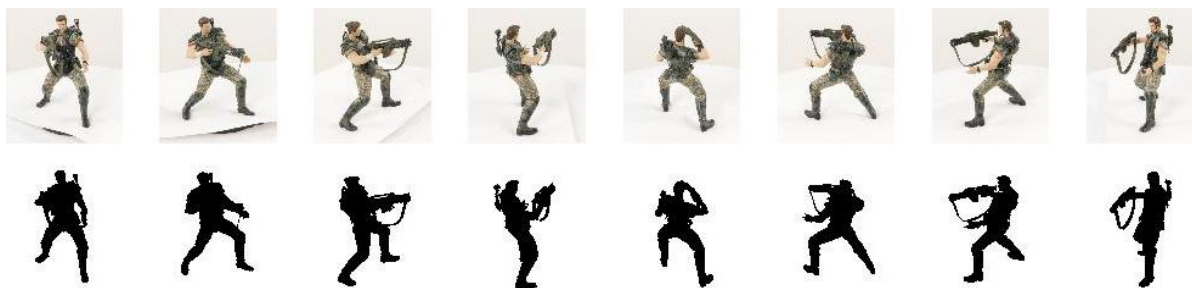
Figure 1: A sample data set: Our system takes as input a set of calibrated images and silhouettes and produces a textured polygonal model (VGG, 2008).
