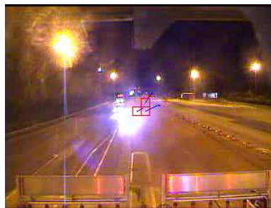
Figure 6: Example of false alarm due to the aperture problem. The optical flow vector are normal to the light beam edge giving completely wrong results.
