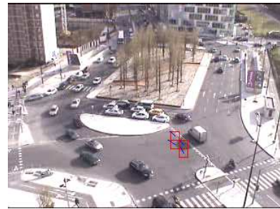
Figure 7: Example of false alarm due to projected shadow. The shadow expands on areas where no movement from down right corner to up left corner are never seen.
