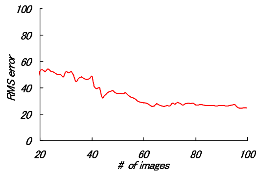
Figure 7: Accuracy of generated arbitrary light source images under the noise in image intensity. The horizontal axis is the number of images used for estimating the intensity projection matrix, and the vertical axis is the RMS error of generated images.
