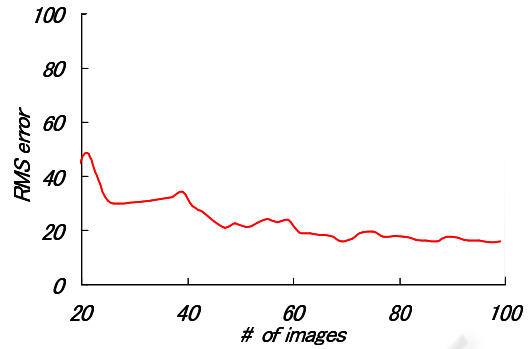
Figure 6: Accuracy of generated arbitrary light source images under the noise in light source positions. The horizontal axis is the number of images used for estimating the intensity projection matrix, and the vertical axis is the RMS error of generated images.
