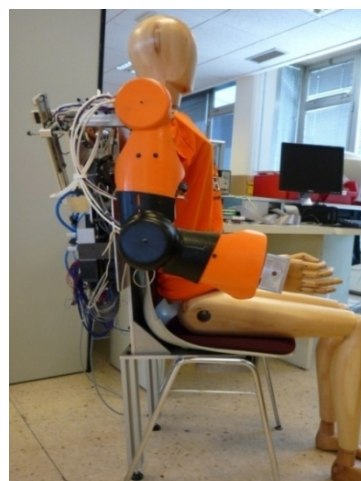
Figure 1: Exoskeleton ÍKO (IKerlan's Orthosis) worn by a dummy.
