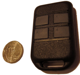
Fig. 2. Wearable sensor for wireless remote identification system.
