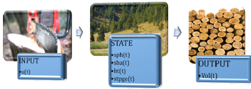
Figure 1: State space representation of the forest stand model, where, t = time in years; sba = stand basal area in m^2ha^{-1} ; ht = stand mean height in metres; stpge = dimensionless stumpage; u = number of trees harvested in stems ha^{-1} ; and sph = initial or residual stand density in stems ha^{-1} .
