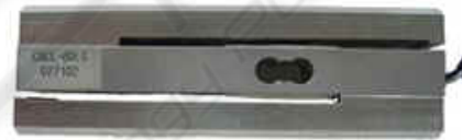
Figure 3: A prototype sensor using load-cell.
