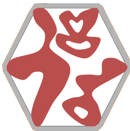
Figure 2a: A 2D example for tunnels and pockets detection composed of three connected components (in brown). The closed curve in black corresponds to the convex hull, and the border B_{CH} in gray embodies the area under analysis and is the starting set of voxels for the propagation process.
