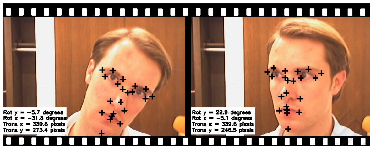
Figure 4: Features tracked by our algorithm. The information box shows rotation and translation parameters.
