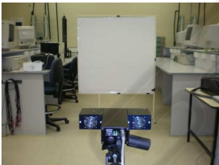
Figure 6: Picture taken from a normal 2D camera for a tripod mounted TOF camera setup.
