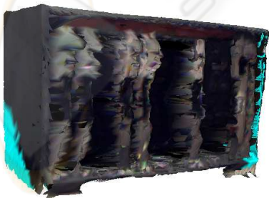
Figure 7: Top: Industrial object with metallic surfaces which are difficult to measure reliably with a time-of-flight camera. Center: Reference 3D Model. Bottom: Reconstructed 3D Model.
