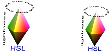
Figure 1: (a) Representation of the hue and saturation components of the HSL color space. (b) Chromatic plane of the HSL color space ( \vec{c}^a and \vec{c}^b represent the projection of two color pixels on this plane).
