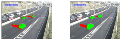
Figure 7: (a) Weak CNCC Classifier results. (b) Weak Classifier + MRF results.
