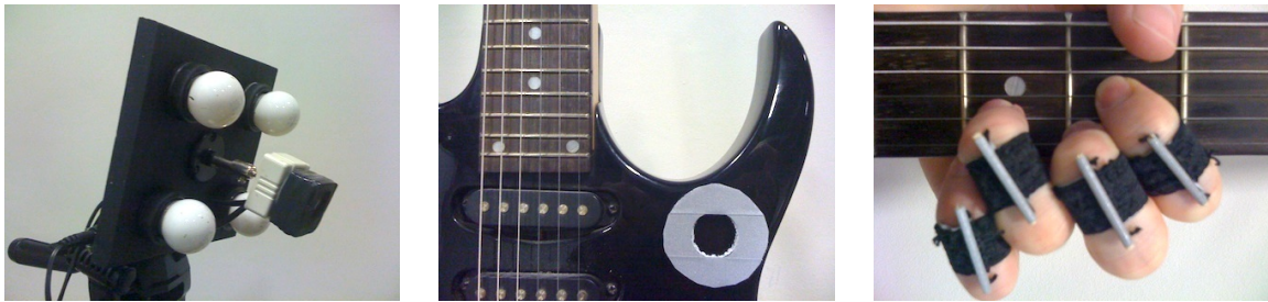
Figure 1: Capture hardware. On the left, an infrared camera surrounded by four infrared light sources. In the center, a hollow disk made with reflexive material. Four of them are used to locate the plane containing the ROI. On the right, middle-phalanges gloves with small rods coated so as to easily reflect light.
