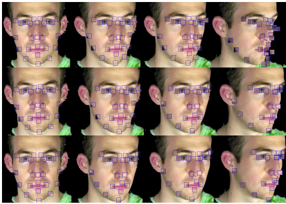
Figure 9: Each row consists of a set of selected frames from a tracking sequence with the synthetic texture patches drawn on which indicates the location of the features. The results at the top are from the single-view approach, at the middle are from the multi-view CLM using shape PCA approach and at the bottom are from the multi-view CLM using shape PGA approach. When the rotating angle reaches certain degrees(b,c), the algorithm continues tracking the face well by auto-switching the appearance model to a side view model while the patches start getting off the position with single-view model.
