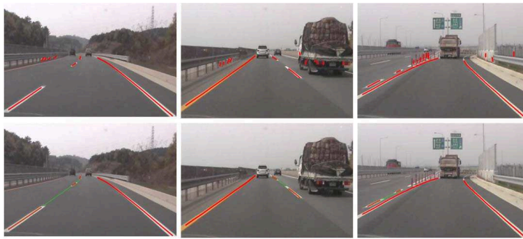
Figure 5: Lane aggregation. The first row: without lane aggregation. Second row: with lane aggregation.
