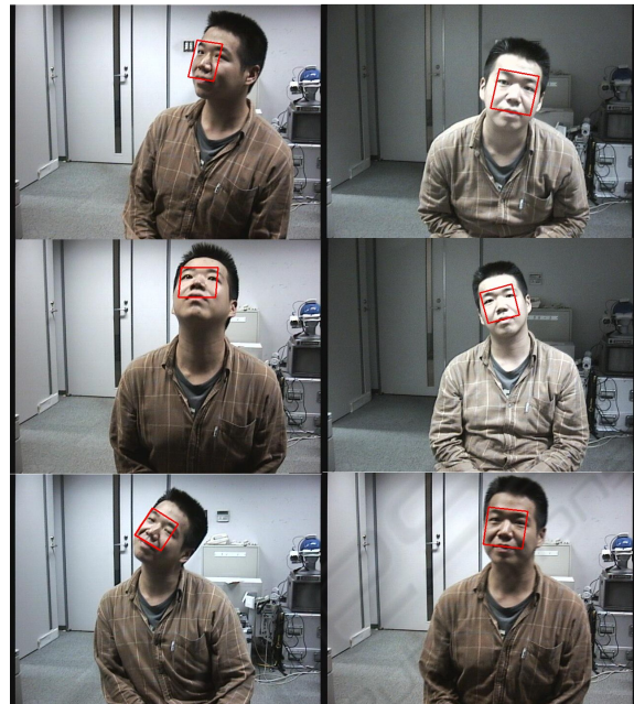
Figure 8: Examples of face tracking results. Red rectangle depicts SLLiP tracker aligned on human face.
