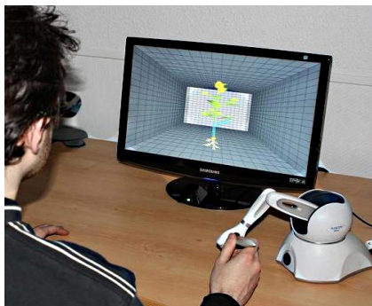
Figure 10: A user working on a virtual plant, with Phantom Omni device, force feedback and stereoscopic viewing.
