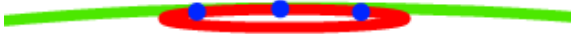
Figure 2: Green: part of the correct ellipse, blue: P_i , red: derived model evaluated in a RANSAC-iteration. It scores a high fitting factor but does not fit the contour well.
