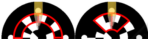
Figure 6: Left: bad layout (2 symbols), recovery not possible. Right: good layout (2 symbols), recovery possible.
