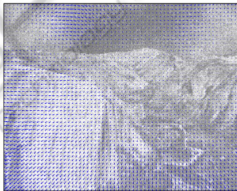
Figure 6: Temporal regularisation. We added Gaussian noise with standard deviation \sigma = 40 to the "Yosemite" sequence. The shown high quality optical flow field is obtained by the control based optical flow approach (4) - (5) (parameters: \alpha = 0.05 and \beta = 0.000003 ).
