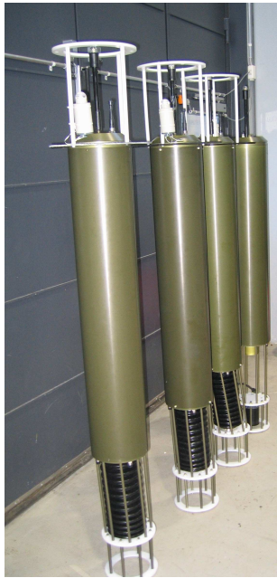
Figure 4: Available physical floats (own by SWARM consortium). Floats are around 2 m tall and weigh approximately 40 kg.
