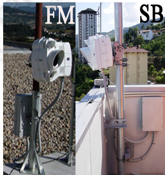
Figure 2: View of the laser heads at FM (Pole III) and SB (Pole II).
