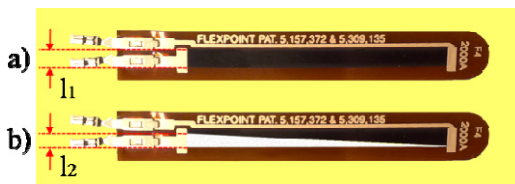
Figure 6: (a) Regular (uncut) geometry sensor, (b) changed (cut) geometry sensor.
