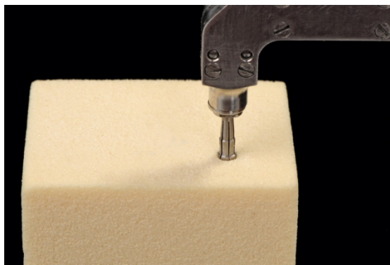
Figure 6: Application of the bone quality testing device in a polyurethane foam model. Following implant site preparation, the sensing element is inserted in the osteotomy and opened gradually both in the cervical and apical part of the socket while the force needed for opening the sensor is measured.
