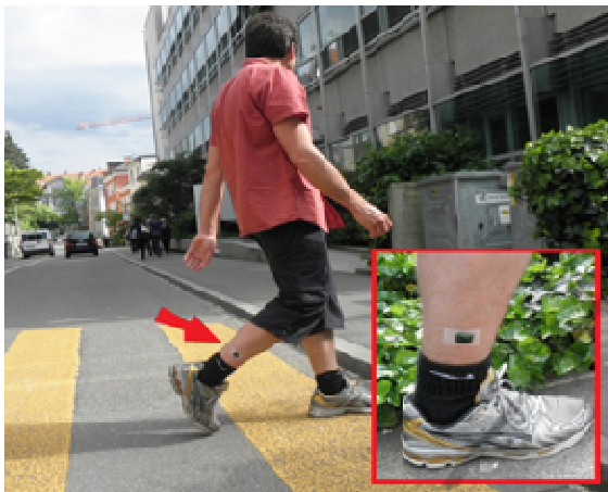
Figure 10: Trial volunteer walking on a road and sensor located against right lower leg.
