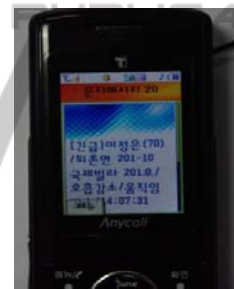
Figure 10: Short message on cellular (Message says, [Emergency] Name(Age)/ Address/ Lower Breath rate/Reduce motion/Time )
