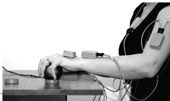
Figure 1: MTx sensor positions on the torso, shoulder (at the top of the image, under clothing), upper arm, lower arm and hand.
