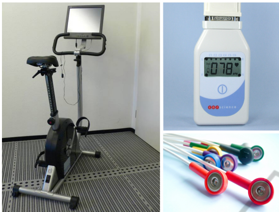
Figure 2: Ergometer bicycle equipped with tablet PC (left), ECG bluetooth sensor developed by the company Cor-science (right top) and body sensors (right bottom).
