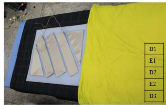
Figure 3: The final design of capacitive textile (silicon pad).
