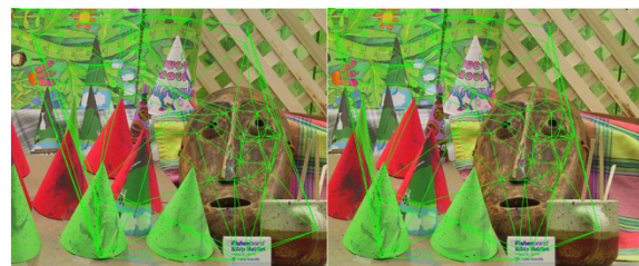
Figure 3: Delaunay triangulation of left and right images using the generated pairs of key points.
