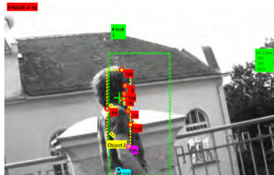
Figure 4: MSaM detection of a moving person (yellow bounding box); Meanshift tracking of person (green bounding box); supporting structure (yellow circles).
