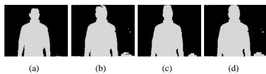
Figure 2: A distance map filtered with different type of thresholding: (a) point with I_y > \lambda ; (b) only set A with \delta = 0.5 ; (c) only set M; (d) set L.
