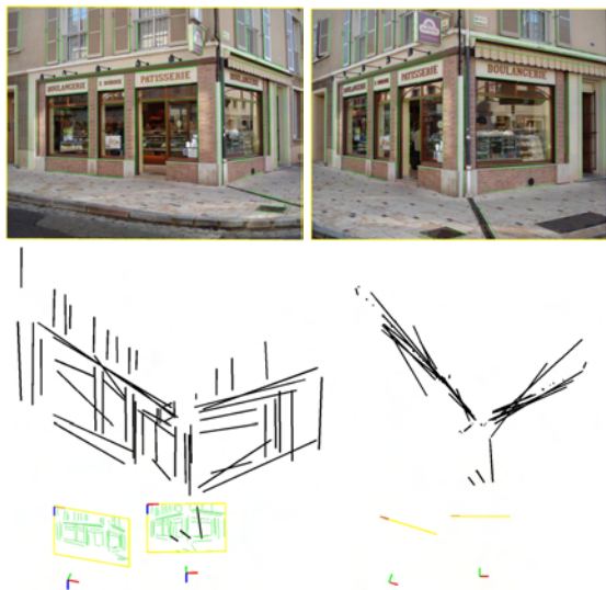
Figure 4: Top row: Two images of a bakery with 85 matched line segments superimposed on the images (in green). Bottom row: 3D reconstruction of the bakery by the structure from motion technique described in (Zhang, 1995). The right image corresponds to the top view.
