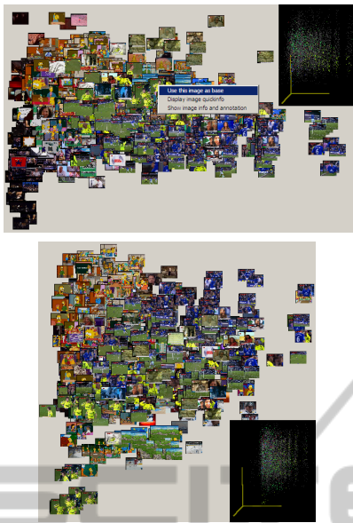
Figure 7: From the current distribution one video is selected (top) as a new base (query) for the new distribution (bottom), which shows the distances of all the videos from the query based on the two selected descriptors.
