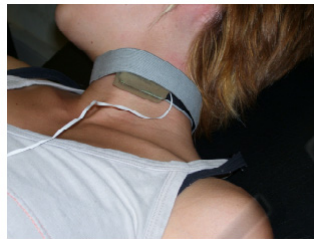
Figure 12: Our probe is held by a collar and placed over carotid artery.
