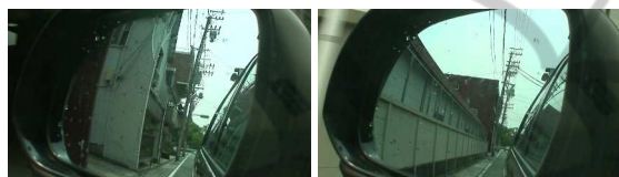
Figure 11: Results of raindrop complement. Comparing these images with those in Fig.10 (a), we find the raindrops are inpainted properly by using the proposed method.
