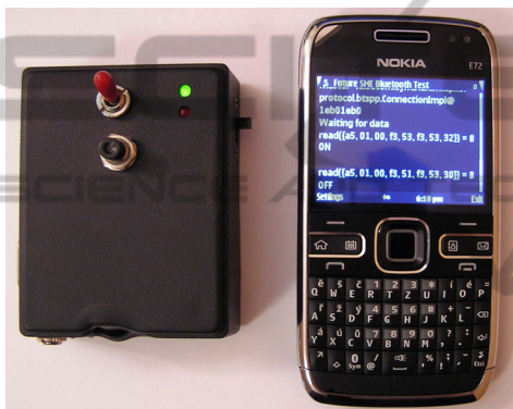
Figure 6: Connecting electronic mobile unit to the F-SME-SPP application.
