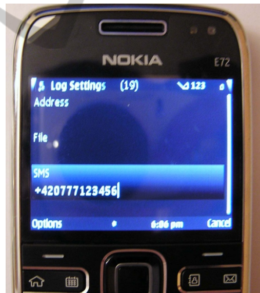
Figure 2: F-SME-GPS application sends SMS with data from an event triggered by the set limit for a in-built accelerometer.
