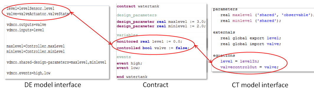
Figure 3: Example of model consistency checking in a water level control system design.
