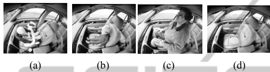
Figure 2: Examples of each of the classes: (a) infant, (b) child, (c) adult, and (d) empty seat.
