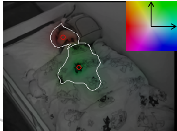
Figure 2: Result after clustering the motion vectors. The red circles indicate the modes of the clusters. The colors indicate here the direction of the motion.
