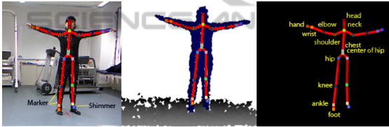
Figure 2: Video Stream (a), Depth Stream (b) and Skeleton rendered in the full body (c) received from Kinect. In (a) and (b) the skeleton is added, in (a) the position of some markers used in MoCap and the Position of one SHIMMER sensor are shown. In (c) the 20 skeleton points are named.
