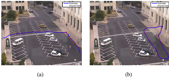
Figure 3: Extracted trajectories using the proposed approach and their corresponding ground truth trajectories.
