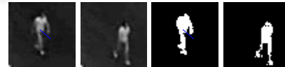
Figure 1: Optical flow between 2 frames. (a), (b) grayscale frames at times t and t+1 , (c), (d) active regions corresponding to the moving person in the two frames.
