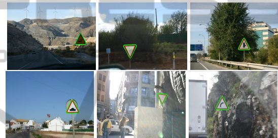
Figure 6: Detection for triangular road signs.
