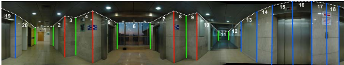
Figure 1: A panoramic image with marked corners and numbered walls. Convex corners appear in green, concave corners in red and flat corners in blue. Note that the user is only required to mark the corners; the orientation and the wall numbering are automatic.
