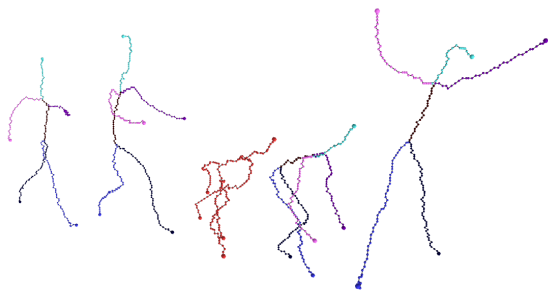
Figure 6: Five frames from the run-crouch-jump sequence (017 from the i3DPost dataset) illustrating the problems that occur when the subject is crouching and no reliable skeleton can be extracted, but also that the algorithm recovers when the arms and legs become distinguishable again.
