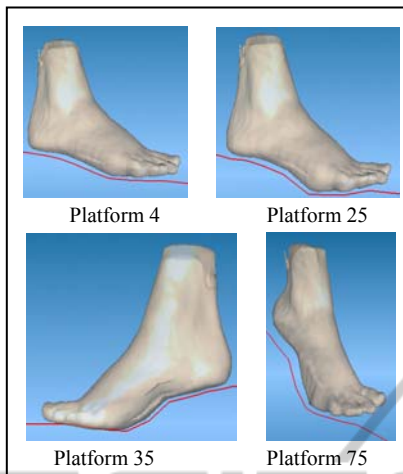
Figure 11: Deformation and inclined platform adjustment of the foot 1 in Figure 10. The deformation line is the red line.
