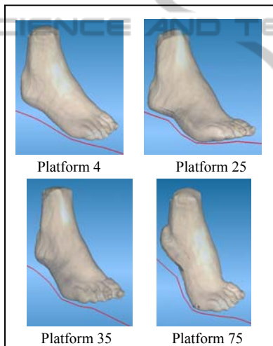
Figure 12: Deformation and inclined platform adjustment of the foot 2 in Figure 10. The deformation line is the red line.
