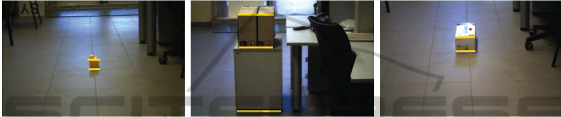
3.4: Actual height is 8.1 cm, estimated height is 8 cm, and \beta = -10^\circ . 3.5: Actual height is 29.6 cm, estimated height is 29.1 cm, and \beta = -15^\circ . 3.6: Actual height is 12.3 cm, estimated height is 11.4 cm, and \beta = -20^\circ .
