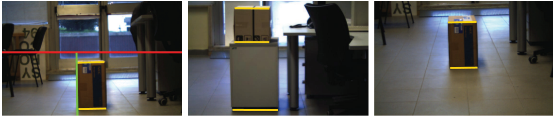
3.1: Actual height of the object is 36 cm, estimated height is 36.3 cm, and \beta = 0^\circ . 3.2: Actual height is 29.6 cm, estimated height is 29.9 cm, and \beta = -7^\circ . 3.3: Actual height is 36 cm, estimated height is 35.7 cm, and \beta = -10^\circ .
