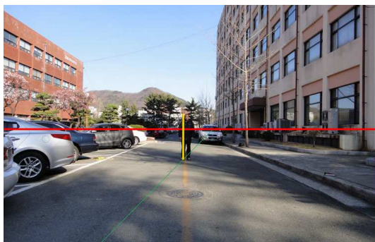
Figure 4: Actual height of the person is 176 cm, estimated height is 175.6 cm, and \beta = 0^\circ .
